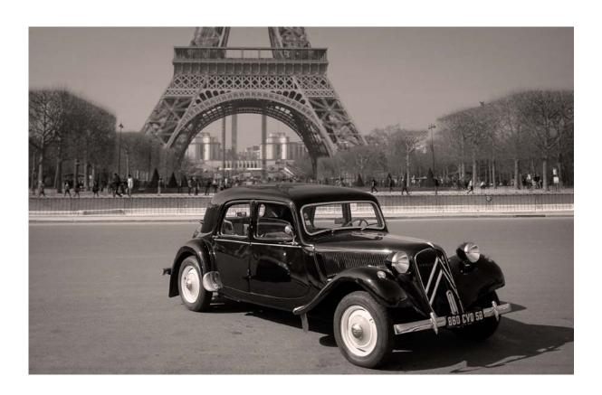
It is difficult to overestimate how important the Traction Avant was: the car you're driving today is based on it. Virtually all previous cars were based around horse-drawn carriages, with an engine and steering added. The all-steel Avant was light, yet strong, small, yet spacious, drove the front wheels, like a modern car, and above all, handled like a car, rather than a carriage.
