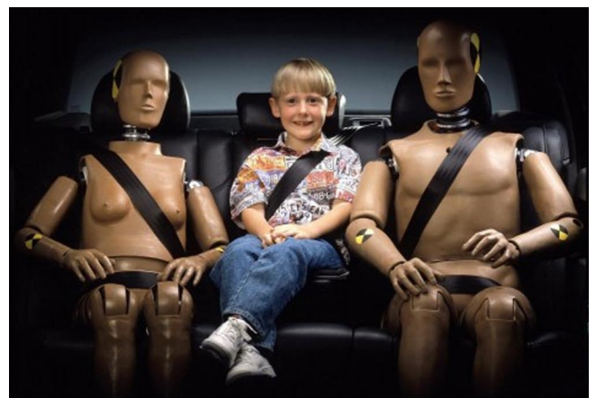
Three-point (also known as lap/shoulder and lap/sash) seatbelts save lives. Note that the child in the picture above is in a booster seat, which helps the belt fit properly.
