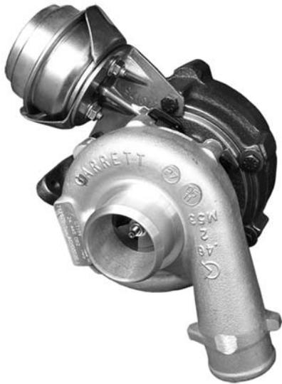
**S**uperchargers & turbochargers are air pumps that look & work rather like a hair drier. They force air into an engine, which makes it work more efficiently and therefore go faster.
